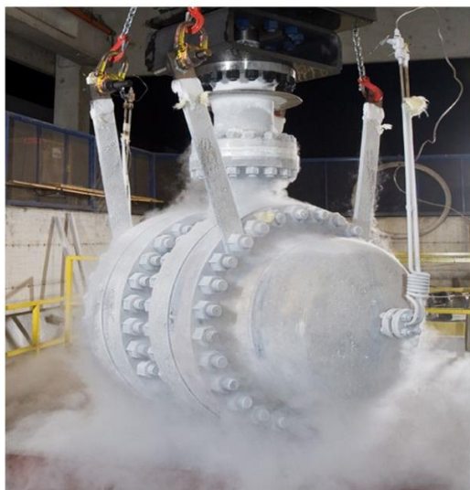
Vanessa™ automated valves from Emerson are designed for cryogenic applications. They are intended to ensure safe, leak-free shut-off during demanding unloading processes. Source: Emerson
