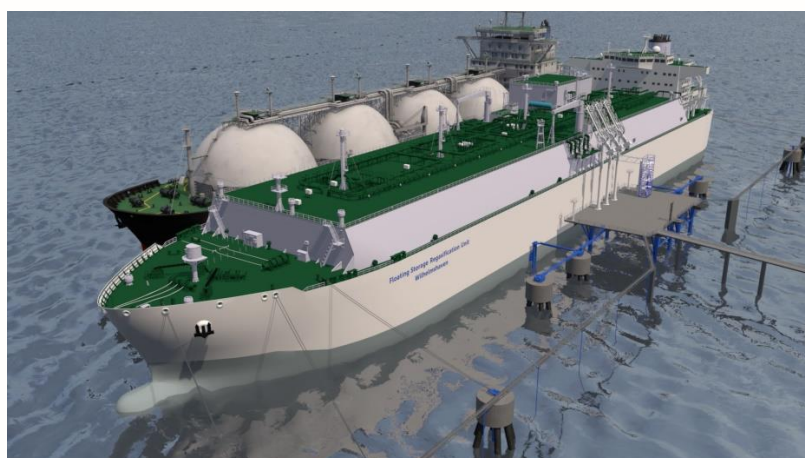
LNG moves Germany: A floating LNG landing terminal – "Floating Storage and Re-gasification Unit" (FSRU), as planned for Wilhelmshaven, is the most economical and quickest way to implement from the point of view of LNG Terminal Wilhelmshaven GmbH. Source: LNG Terminal Wilhelmshaven GmbH
